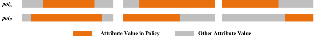
Fig. 3. Three types of conflicts between different policies: cover (left), overlap (middle), non-overlap (right).
